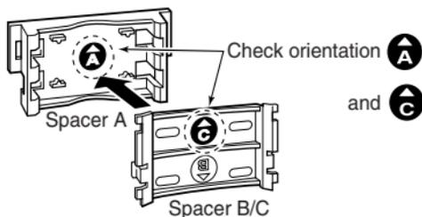
**NOTE:** Push the notch carefully when remove the spacer from the adapter.
